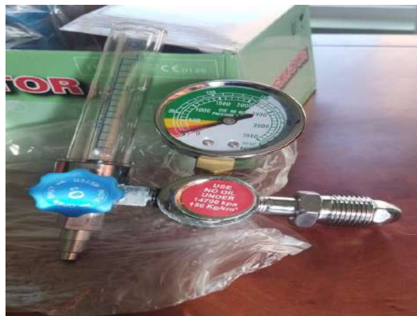
Figure 3.5: Gas flow meter.
