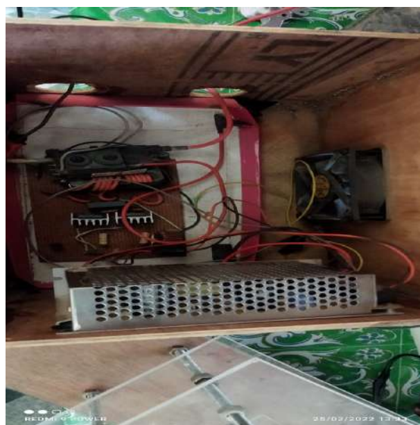
Figure 3.6: Power supply made for plasma production in laboratory of CDP.
