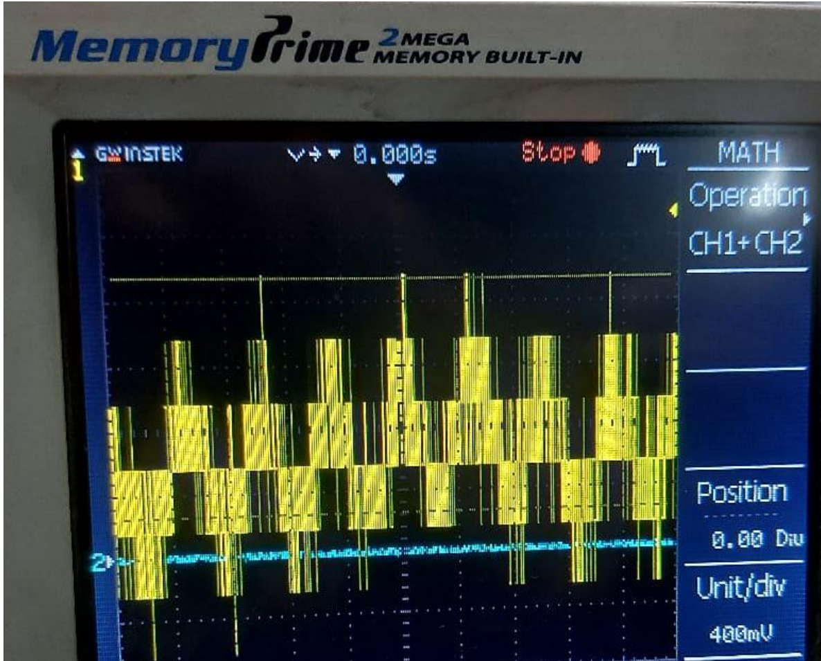
Figure 26: Output waveform of 5 level CHB MLI
