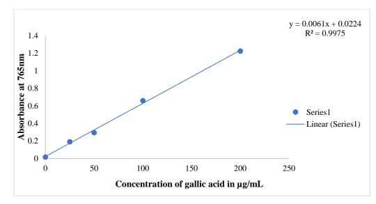
Figure 3: Calibration curve of gallic acid
