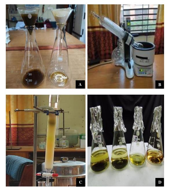
**Figure 2:** Extraction of phytochemicals in 90% Methanol (A); Evaporating solvent with the help of rotary evaporator (B); Sephadex separation (C); Fractionated extracts collected based on the colour band in different vessels (D).
