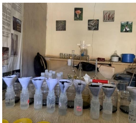
Soil aliquots extraction for potassium
