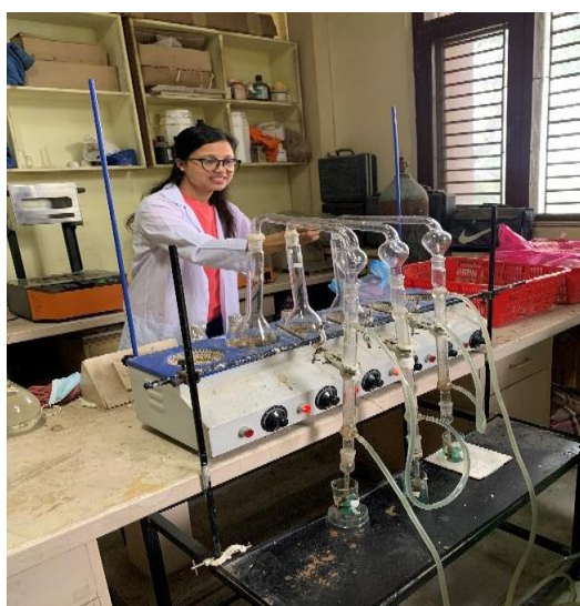
Distillation process of TN
