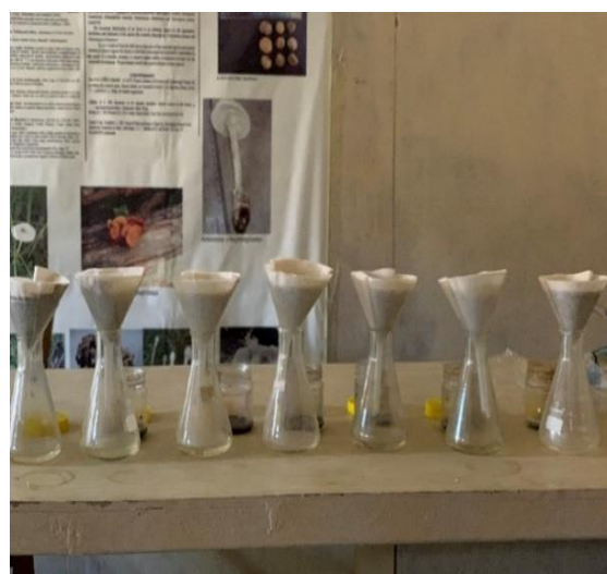
Soil aliquots extraction for phosphorus
