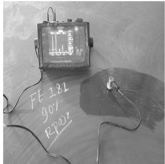
Figure 4.6: Weld joint to be repaired
