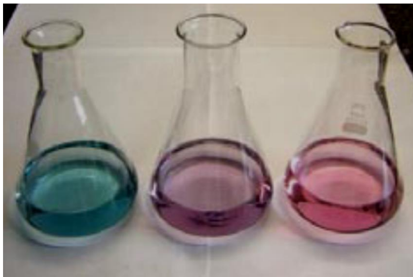
Figure 2.1. Color of solution during EDTA titration in presence of Erichrome Black T indicator.
