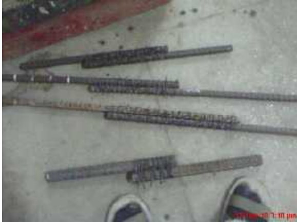
Photograph no 10: Specimens-various lap length
