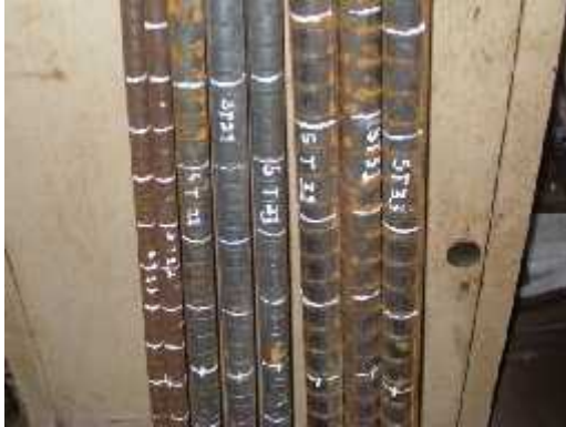
Photograph no.1: Specimens- different \varnothing reinforcement bars
