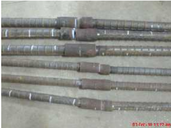
Photograph no 8: Specimens after tensile test.
