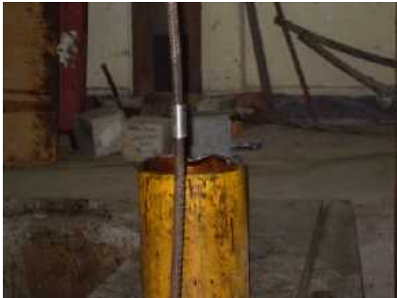
Photograph no 7: Specimen subjected to compression test.
