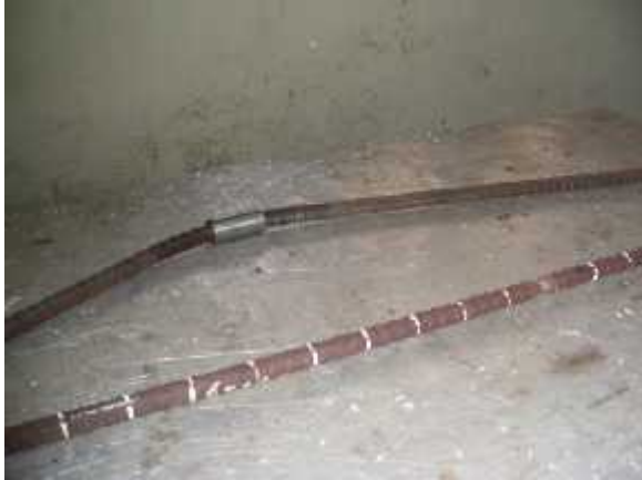
Photograph no 14: Specimens after tension and compression test.
