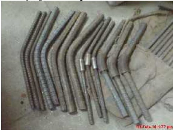
Photograph no 9: Specimens after compression test.
