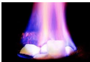
Figure 1: Methane hydrate, in contact with fire, burns upon release of methane. ( https://soundwaves.usgs.gov/2012/06/ dated: Jan 12, 2016.)
