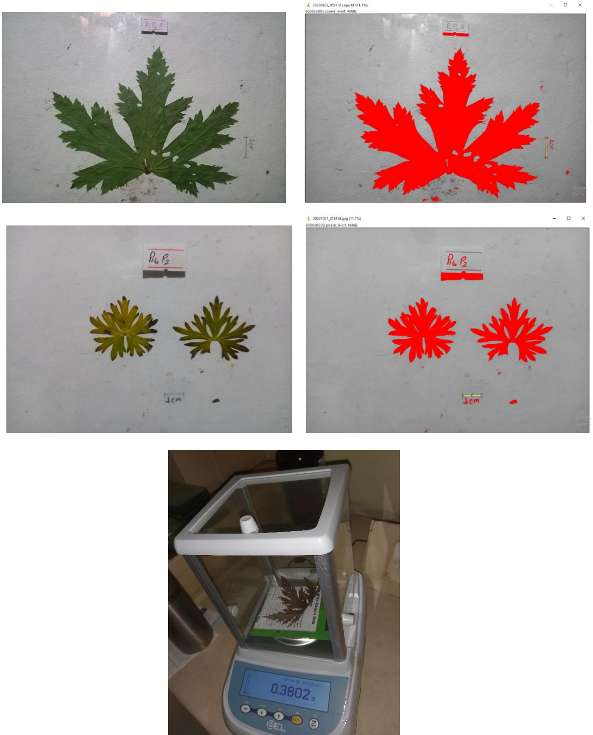
Leaf sample analyzed through image J for determination of leaf area (upper two) and weighing of dry leaf mass (lower one)
