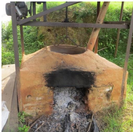
Furnace provided with motor for soya bean roasting
