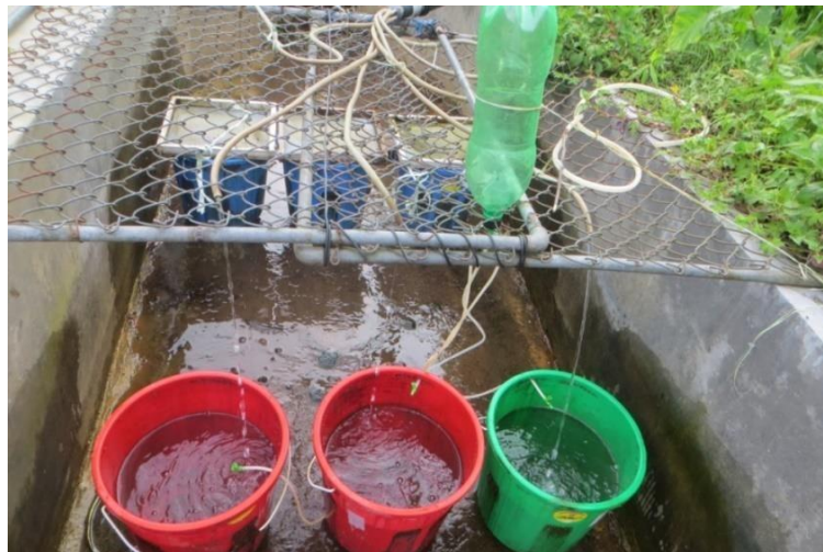
Photograph II: Sucrose solution supplied to each bucket through pipeline
