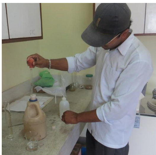
Diluting the hydrochloric acid
