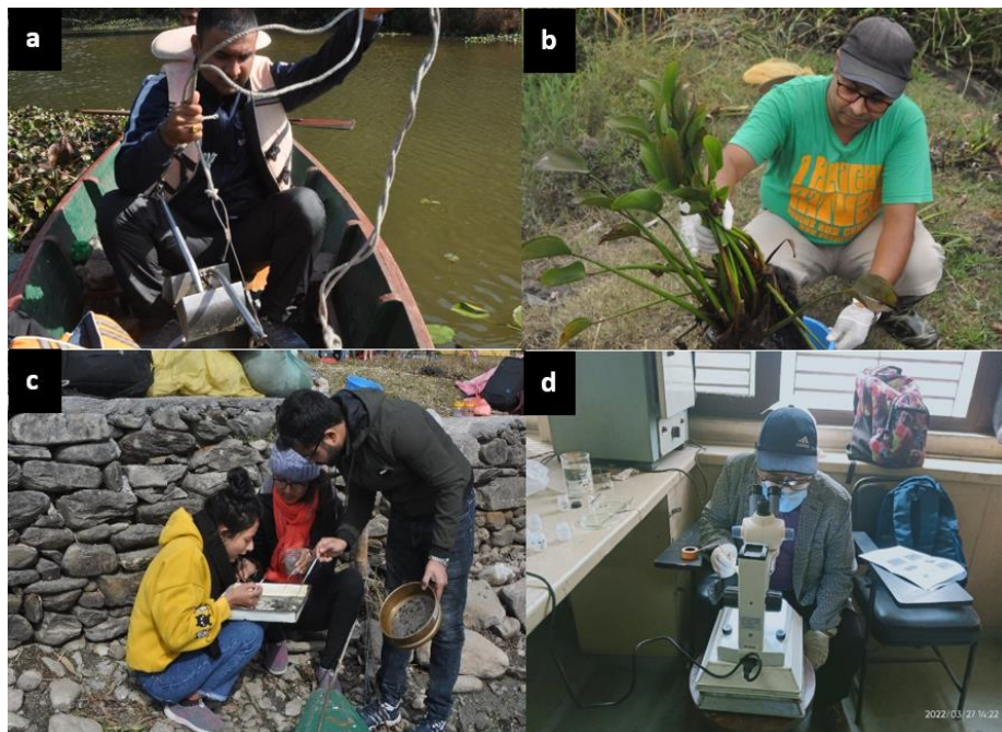
Figure 2: Sampling of macro-invertebrates using Grab Sampler (a), combing of roots of water hyacinth (b), screening of grab samples (c) and identification of macro-invertebrates (d)
