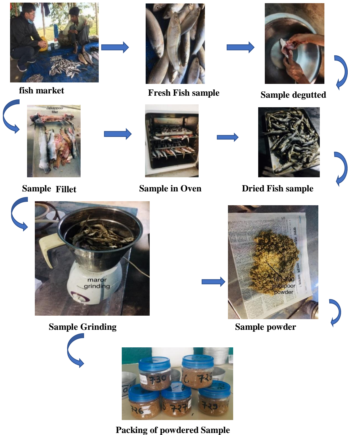
Figure 3: Flow chart of sample preparation of four commercially important fish species for proximate analysis.
