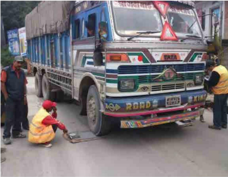
Figure 6.4: Axle Load Survey
