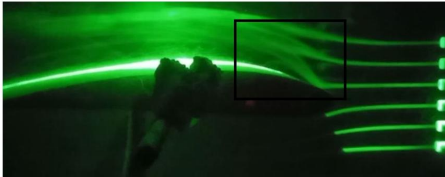
Figure 34: Flow around a highly cambered airfoil
