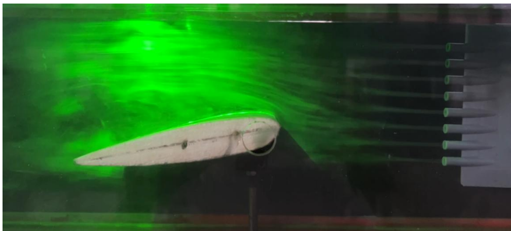
Figure 33: Flow around an airfoil at wind tunnel speed of 1.32 m/s
