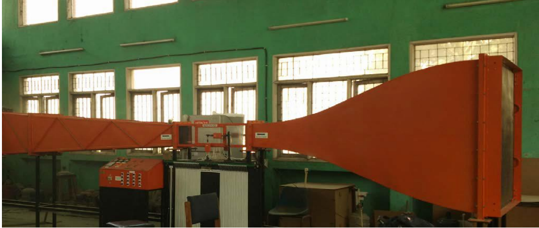
Figure 3:Low speed wind tunnel at Department of Mechanical and Aersopace Engineering
