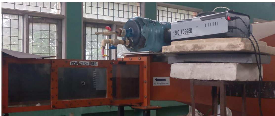
Figure 11: Smoke Visualization Setup
