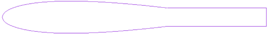
Figure 12: 2d smoke rake profile
