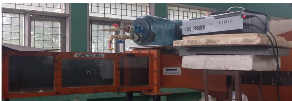
(g) Flow Visualization Setup
