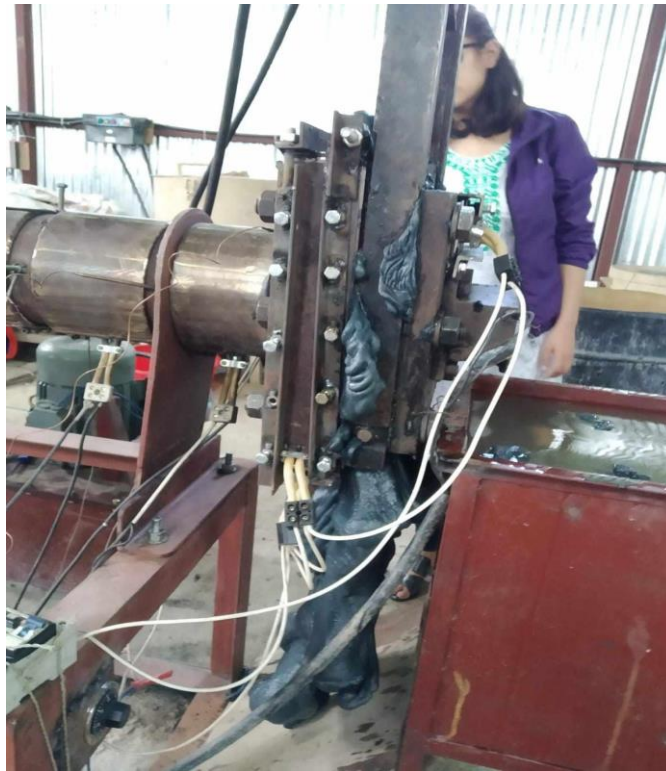
Figure 31 Leakage in hydraulic head system
