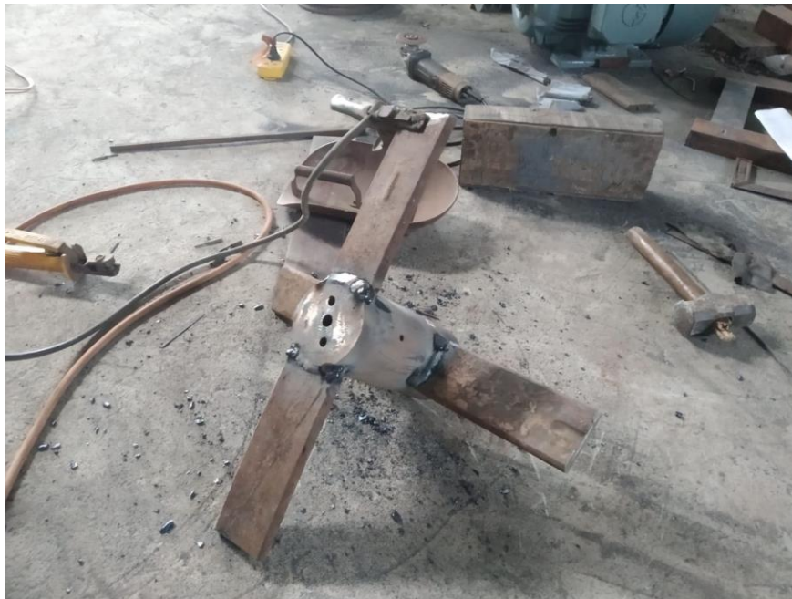
Figure 29 Mixture blades during fabrication
