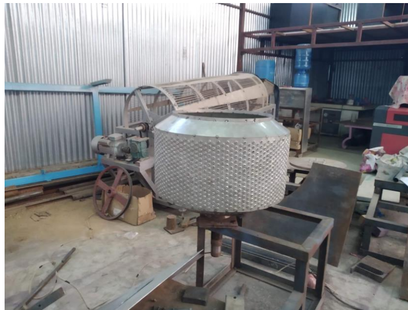
Figure 27 Inner cylinder fabrication
