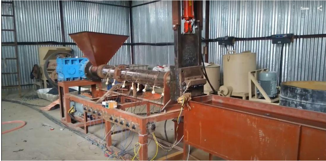
Figure 30 Extruder along with hydraulic head setup
