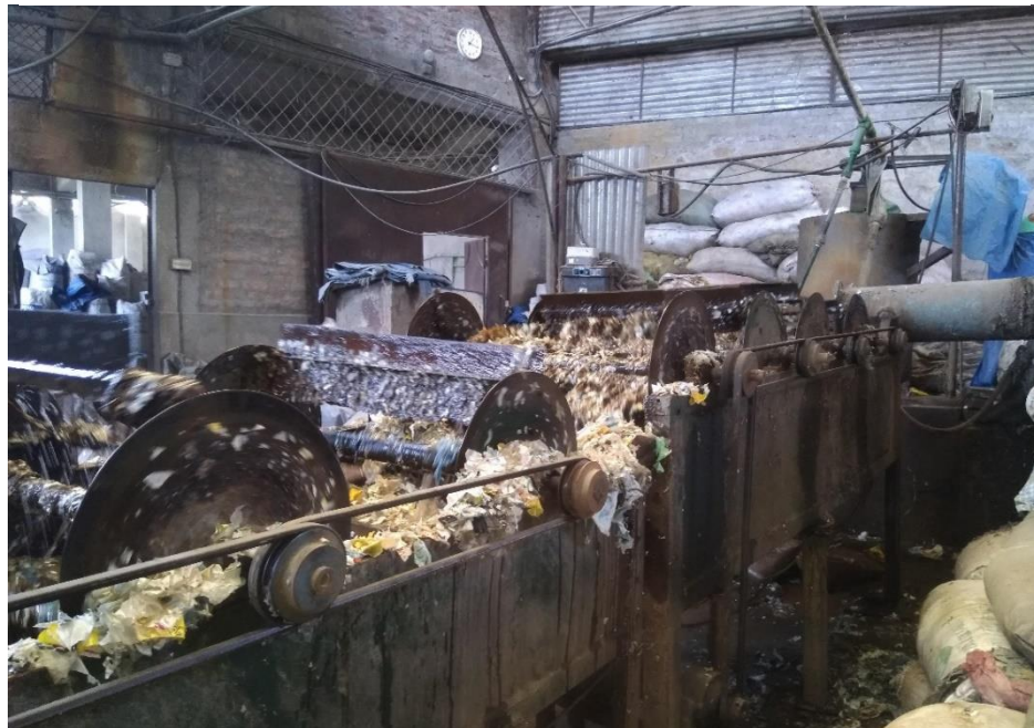
Figure 24 Conveyer washing system
