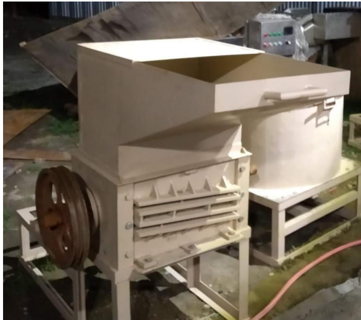
Figure 26 Fabricated granulator machine
