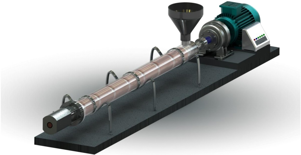
Figure 15 Rendered 3D model of an extruder assembly
