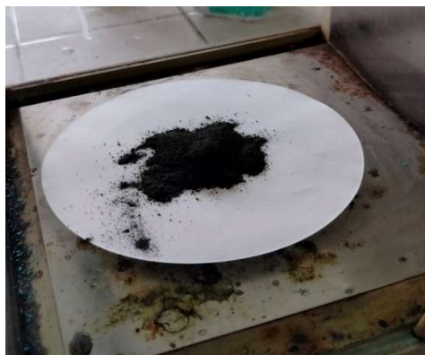
Figure 3.2 Synthesized Copper Oxide Nanoparticle
