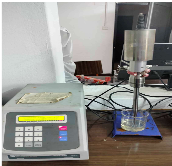
Figure 3.3 Blending of CuO Nanoparticles on ultrasonication machine with ultrasonication of fuel
