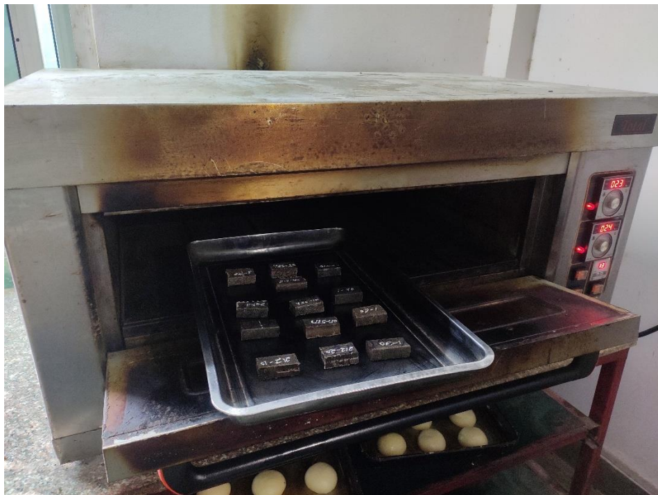
Figure A-6: Drying samples at 105°C for 1 hour
