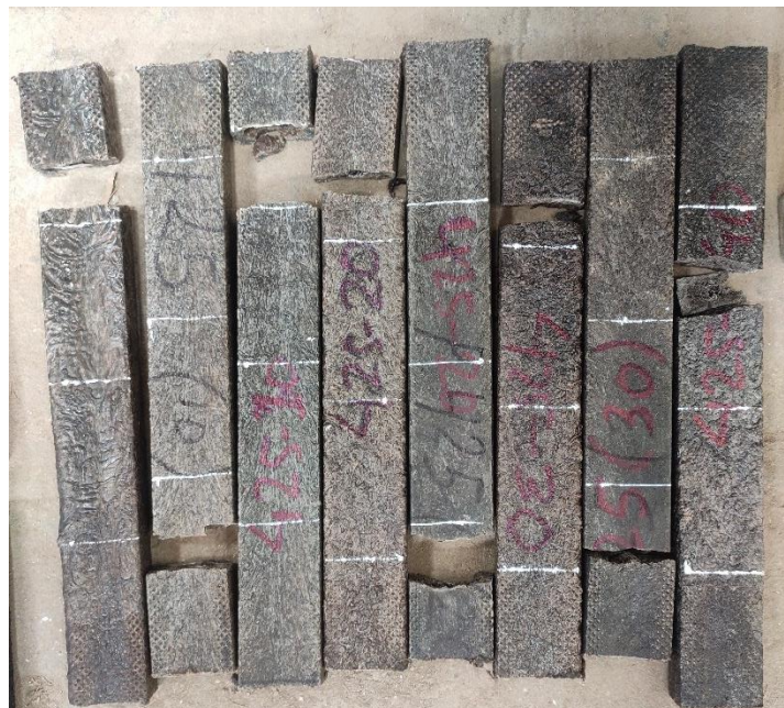
Figure B-2: Test specimens after breaking in UTM
