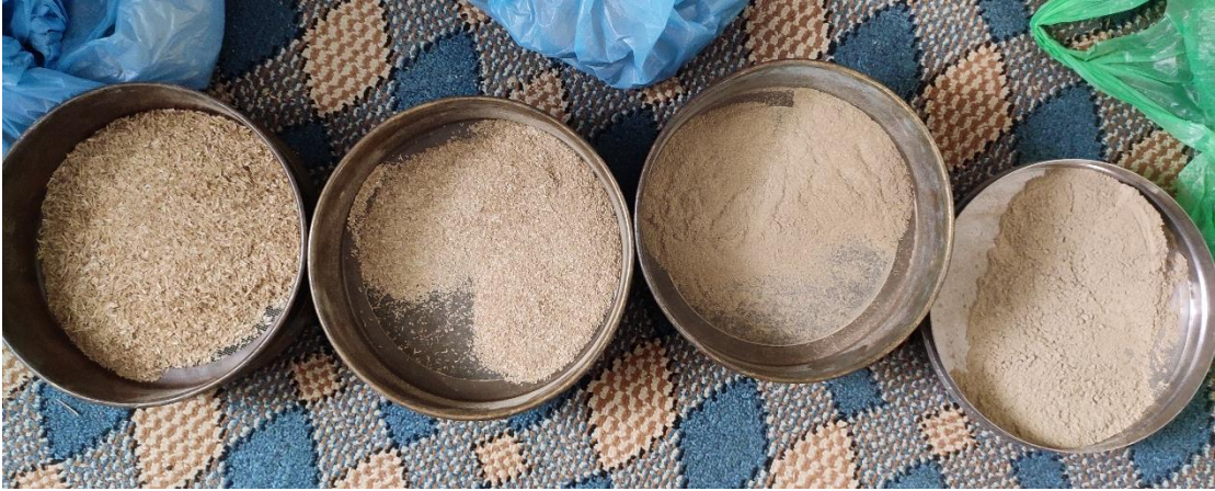
Figure A-7: RH Residue, 1000 microns, 412 micron and 212 microns (from left)
