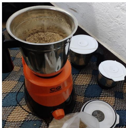
Figure 10: Grinder for making finer RH particles
