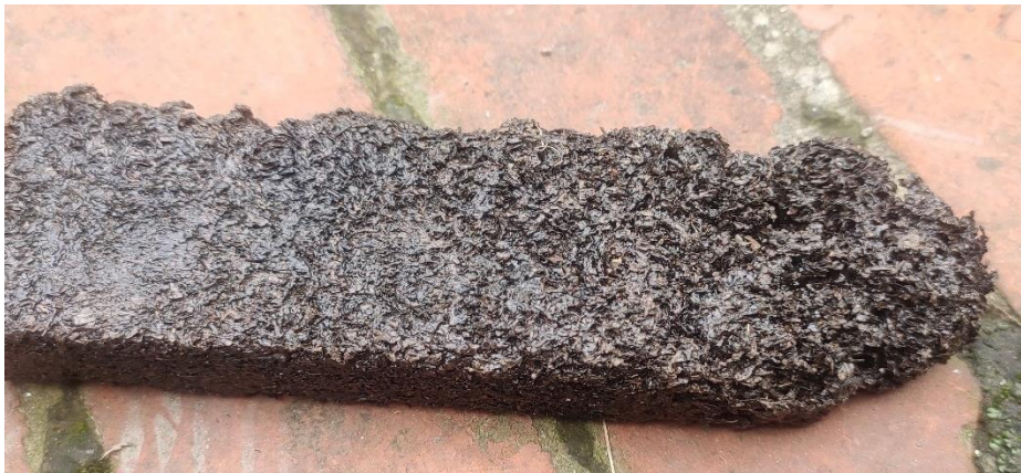
Figure 15: Charred sample due to high temperature
