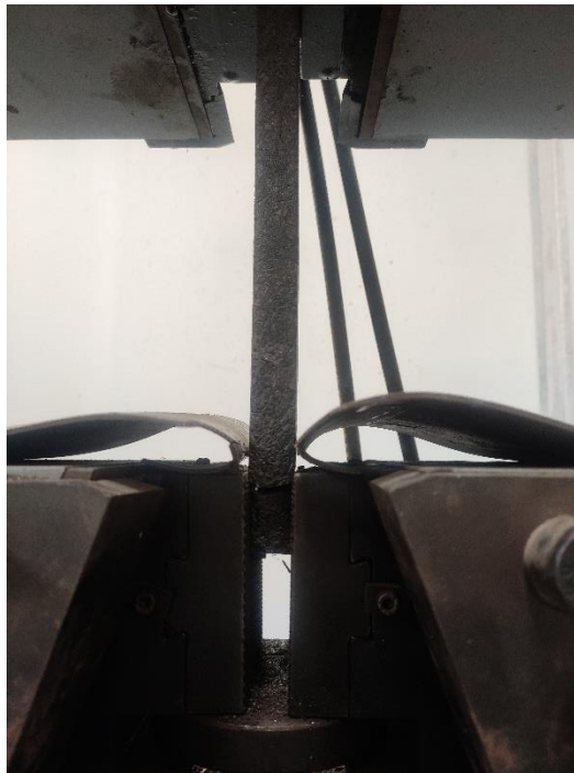
Figure B-4: Clamping specimen with jaws (UTM)
