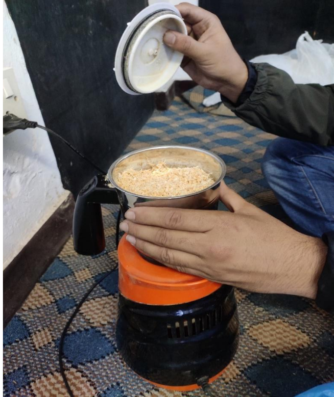
Figure A-1: Grinding filler particles
