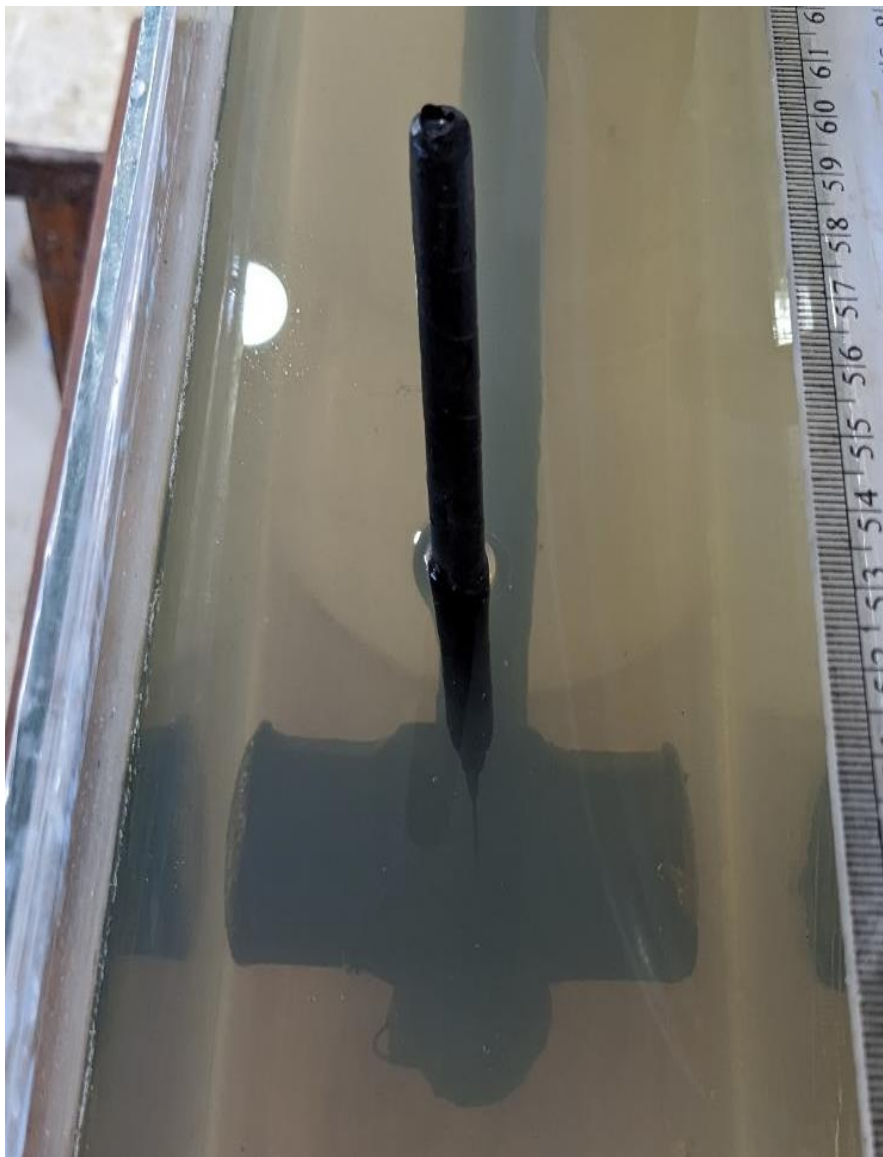
Figure 4.9: VIV turbine model attached to ballast tank
