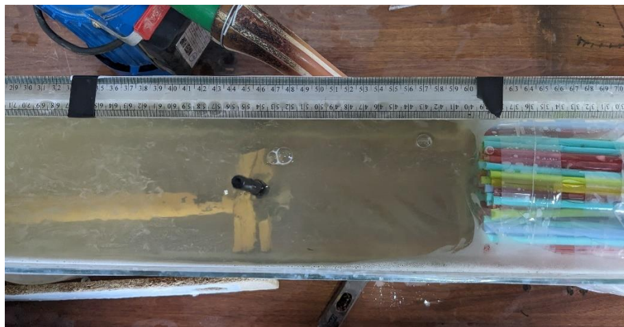
Figure C: Top view of experimental tank showing turbine and measurement scale
