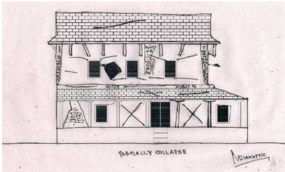
Figure 5.31: Damage Indicator: Partially Collapsed (Large and extensive diagonal cracks in walls, failure of small elements like strut, failure of gable wall, fall down large pieces of mud plaster, fall down pieces of slate from roof and stone pieces from wall, bulge in wall, pillar etc.)
