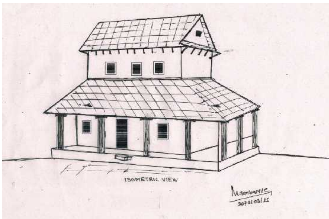
Figure 5.36: Projected roof protects mud plastered wall
