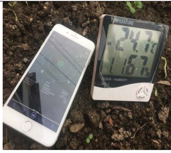
Hygrometer showing temperature and humidity data
