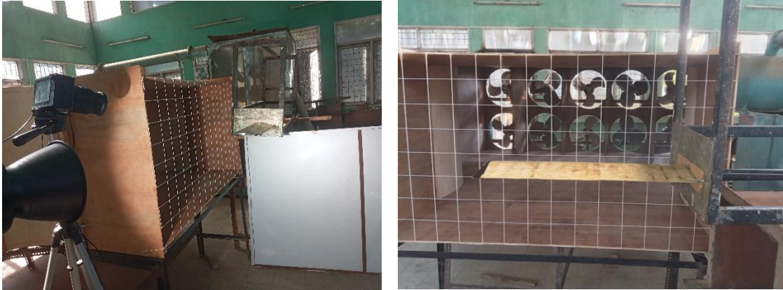
Figure 34 Setup to test Aerodynamic Loading
