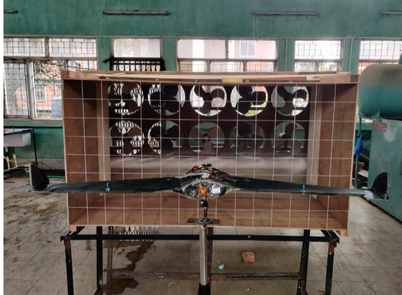
Figure 35 Setup to observe control surface response
