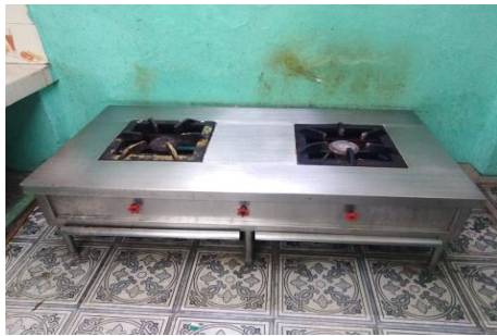
Figure 2: LPG stove with two burners (Overall size: 70 in.×36 in.×20 in.)
