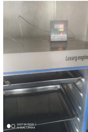
Figure 17: Temperature Measurement at top tray (using PT 100 Thermocouple)
