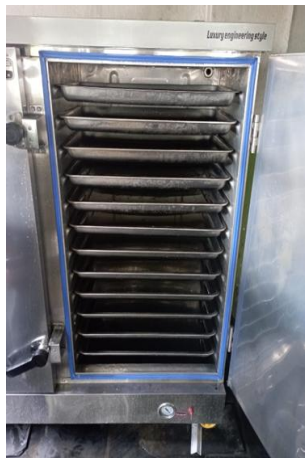
Figure 6: Electric rice steamer (one door open) 12 trays inside one cabinet
