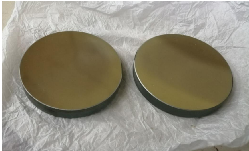
Figure 4.4: Parabolic mirrors of a reflecting type telescope
