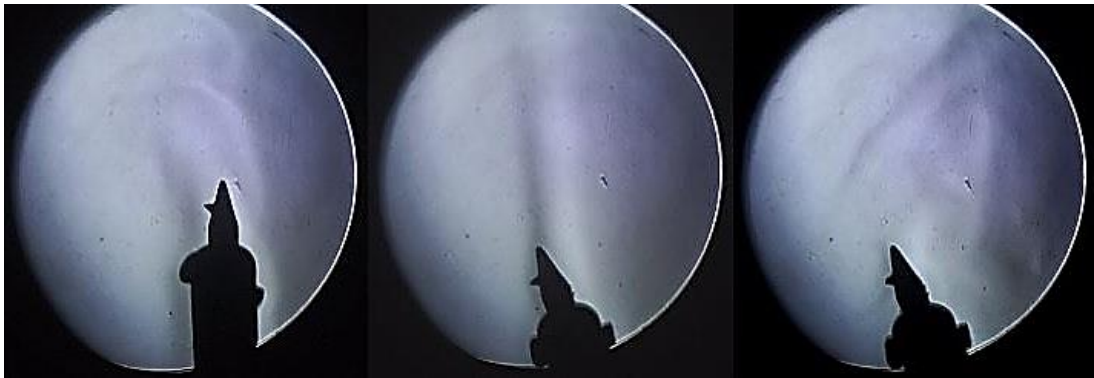
Figure 3.4: Heated air near the periphery of a soldering iron rod rising upwards
