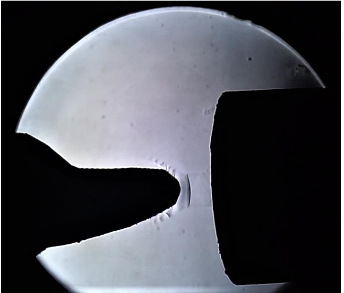
Bow-shock formation in front of the nose of an aircraft model (captured by Sony ZV-E10 Mirrorless Camera)
