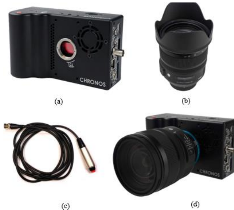
Figure 4.6: Chronos 2.1-HD High speed camera (a) Camera body, (b) Sigma 24-70mm lens, (c) Trigger switch cable, (d) Camera body-lens setup
