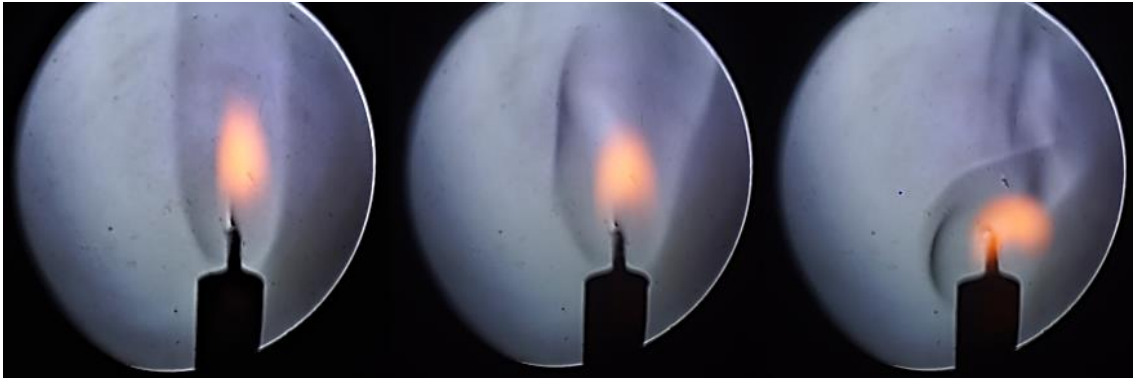
Figure 3.3: Uniform laminar cylindrical flow of a candle plume and its transition to disturbed flow
