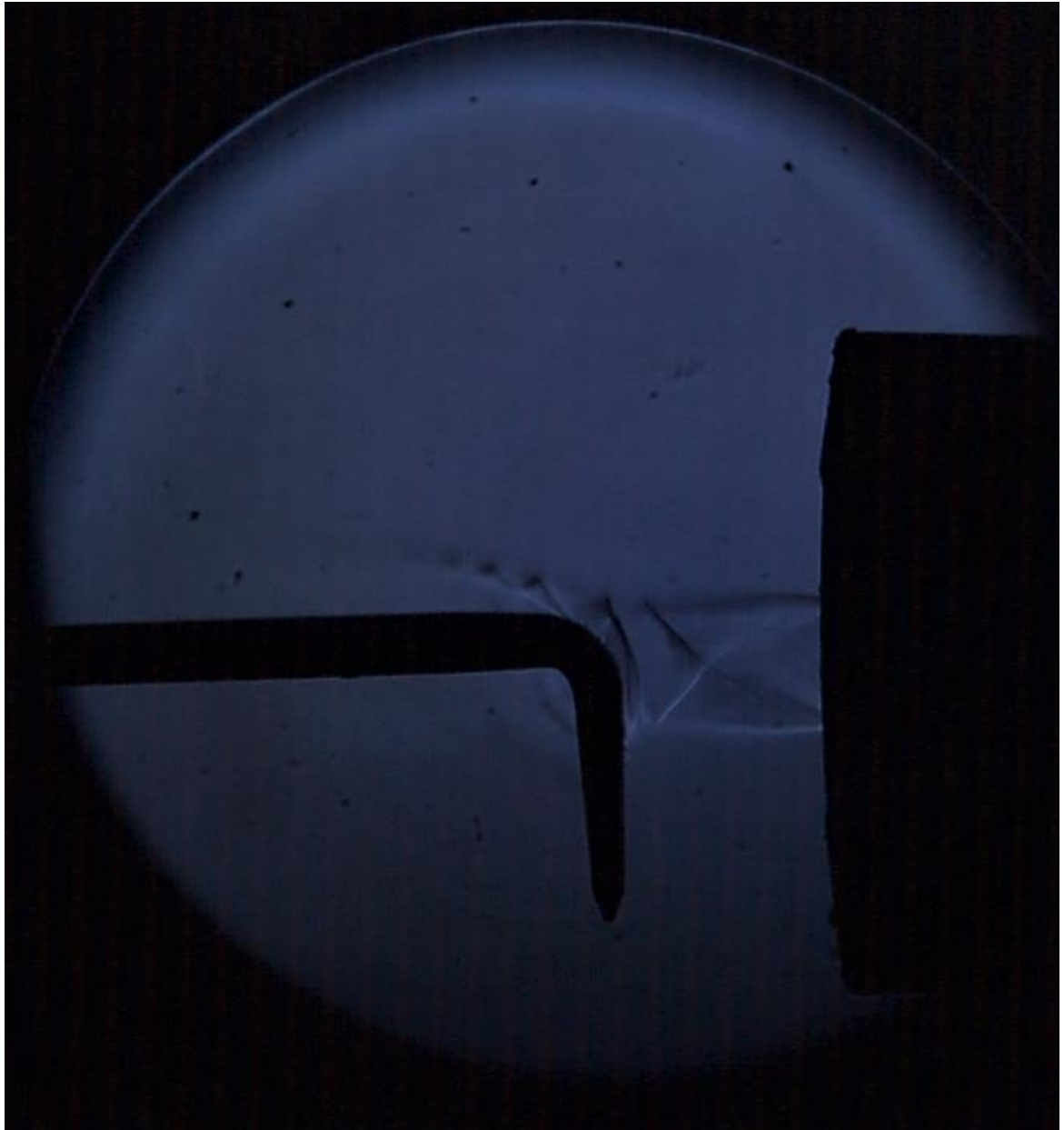
Bow-shock formation in front of the L-shaped blunt body (captured by Chronos High Speed Camera, 1000 fps, 1920×1820-pixel intensity)
