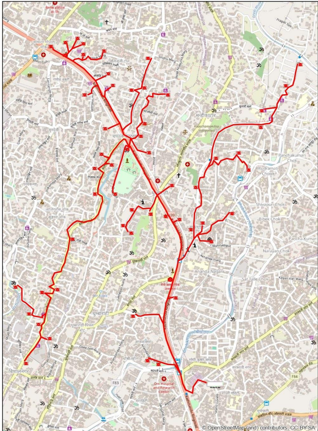
Figure 3.2: Route Map for PEV Travel, OM Distribution Feeder Route and Location of Different Distribution Transformers
