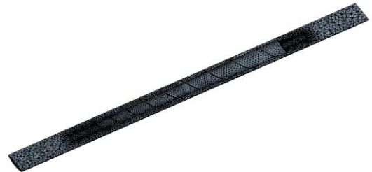
Fluid Domain for variable pitch screw with Straight shaft
