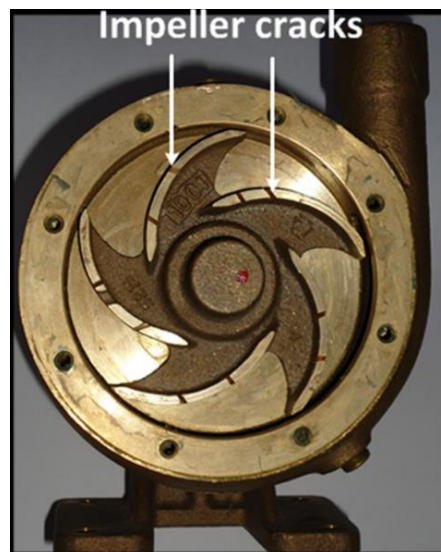
Figure 5: Pump with Impeller Crack used in Rapur et. al (2016)
