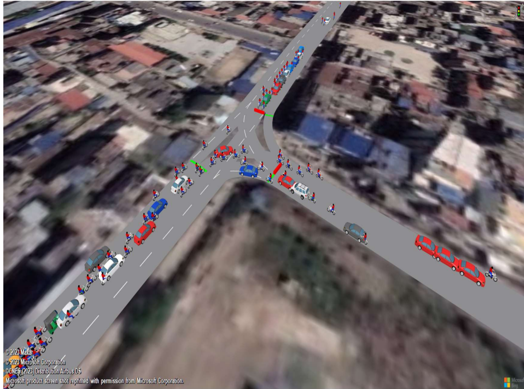
Figure 4-4 Screenshot of the Simulation Run of Padmodaya Intersection in VISSIM (3D Visualization)
