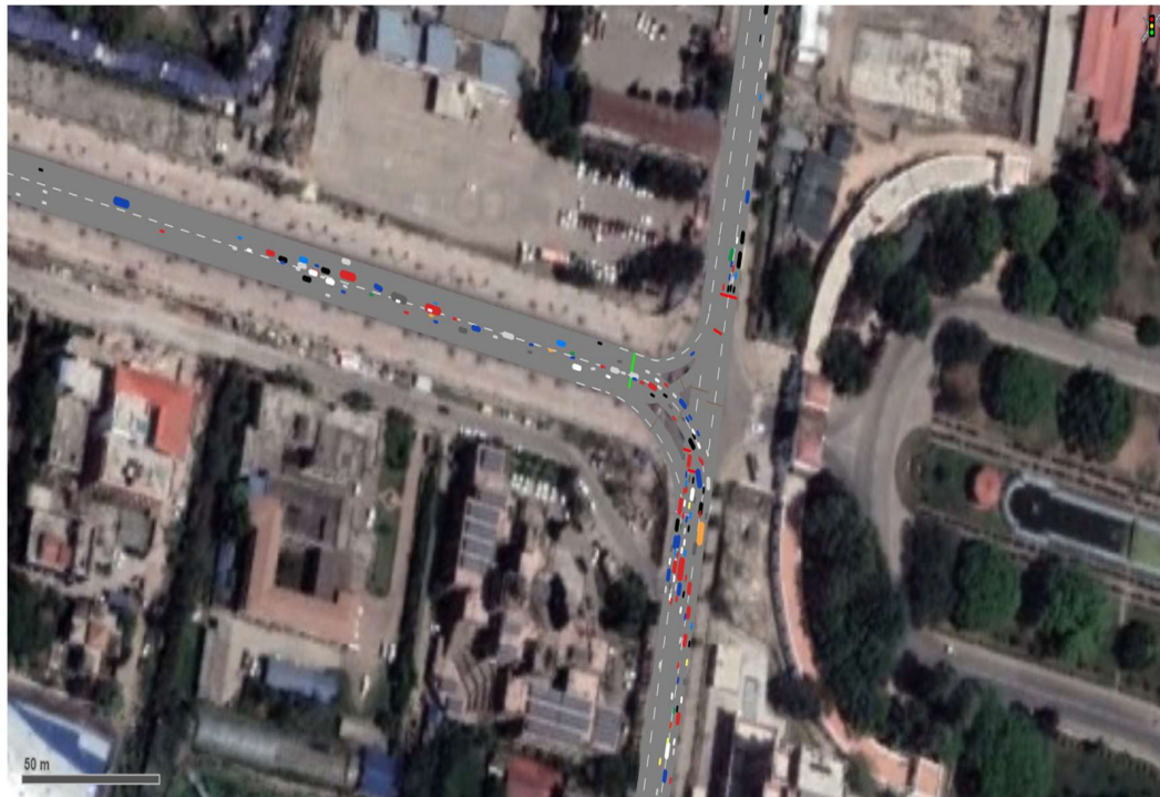
Figure 4-1 Screenshot of the Simulation Run of Singhadurbar Intersection in VISSIM (2D Visualization)
