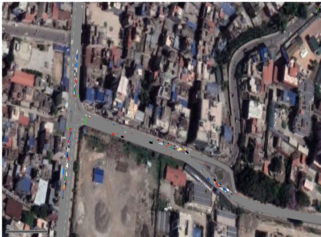
Figure 4-3 Screenshot of the Simulation Run of Padmodaya Intersection in VISSIM (2D Visualization)
