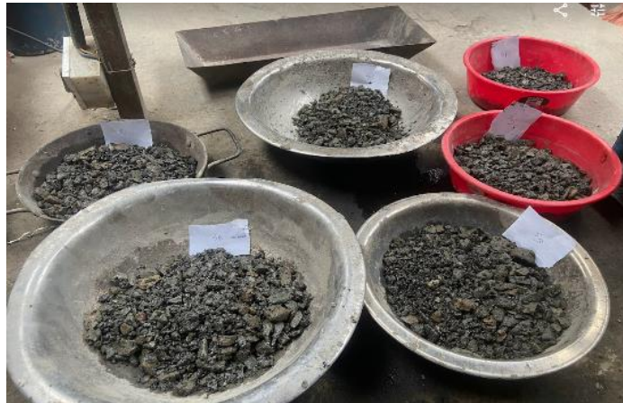
Figure 3.7 Sample after mixing with Emulsion
