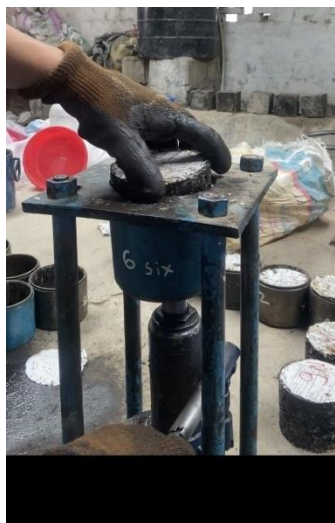
Figure 3.10 Sample Extracting from Mold by Extrusion Jack
