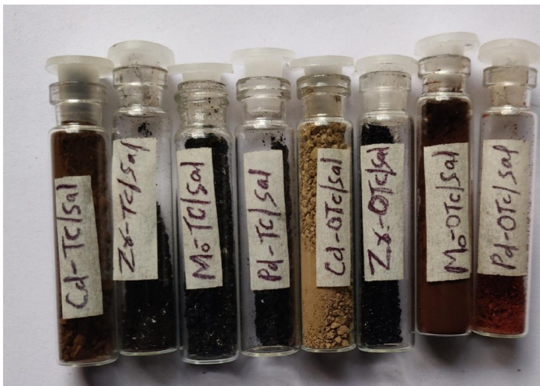
Figure A1: Sample picture of M-TC/Sal and M-OTC/Sal metal complexes.
