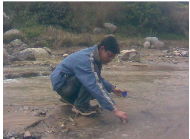
Plate 12: Researcher taking water sample in a vial for faecal coliform test
