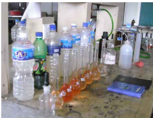
Plate 13: Series of volumetric of flasks made ready to take absorbance for iron
