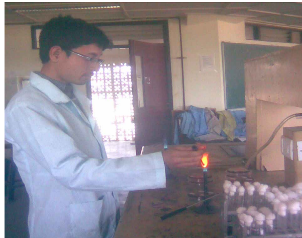
Plate 18: Researcher sterilizing the inoculating loop to perform MPN test for faecal coliform
