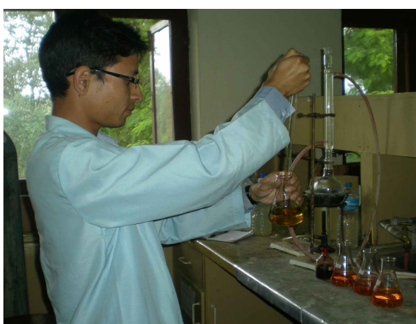
Plate 17: Researcher doing titration for determination of COD
