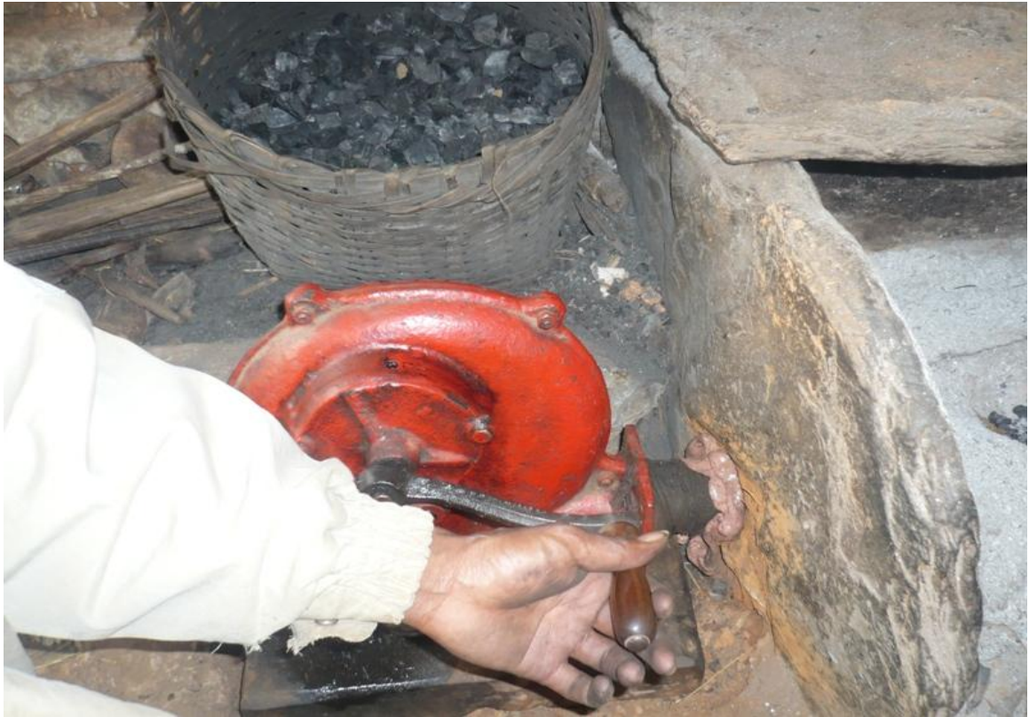
Photograph No. 3 A man is running furnace's Fan,
