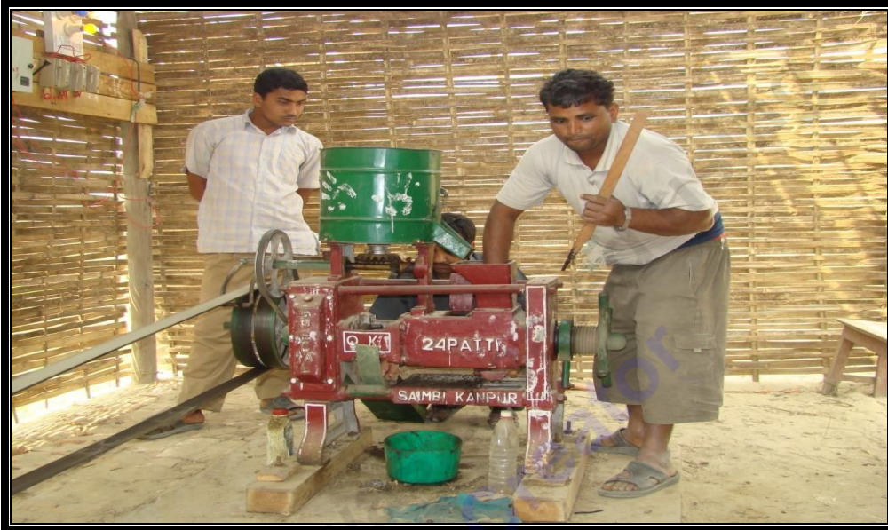
Photo 1: Oil expelling at Siraha district (Source: Adopted from AEPC)
