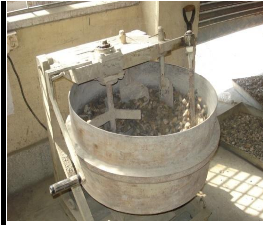
Figure 3.5.1: Plate concrete mixture machine.
