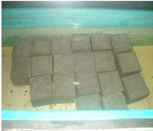
Figure 3.5.3: Thermostat curing tank.
