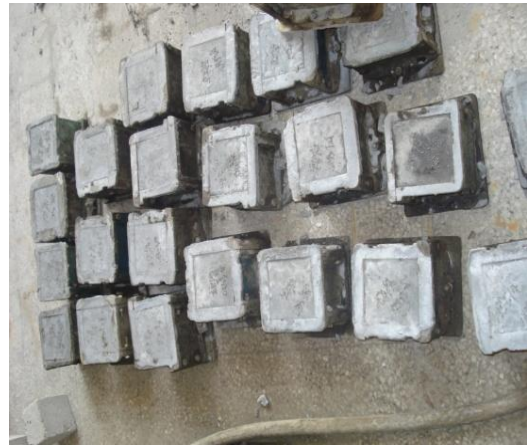
Figure 3.5.2: Mould with specimens
