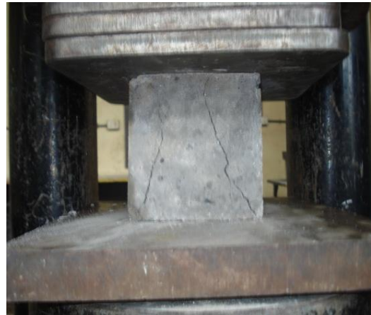
Figure 3.5.4: Compression test on UTM
