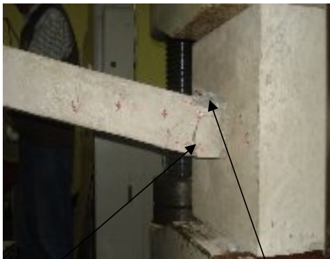
Distinct flexural crack and crushing Of concrete on compression side.
