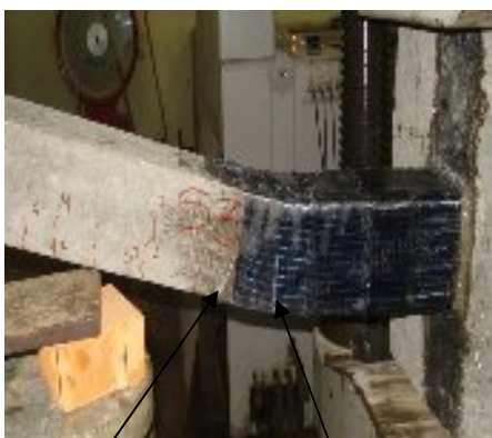
Flexural crack and tearing Of CFRP
