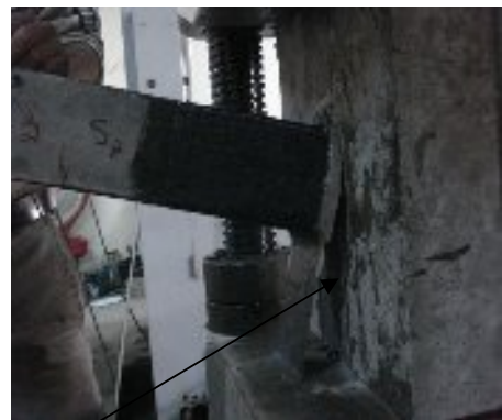
complete delaminating of CFRP
