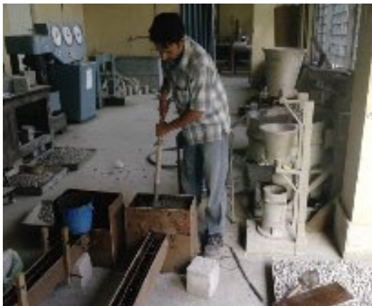
Fig.4, Casting of specimens
