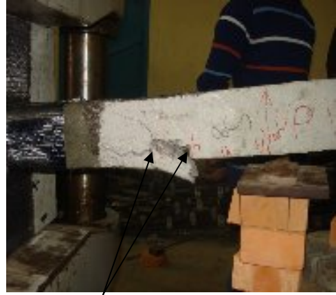
Crack extending towards footing Side and concrete spalling.
