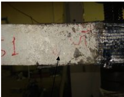
Flexural crack above CFRP wrap
