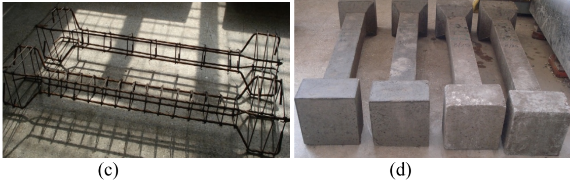
Figure: 3.8 Detail of Casting Group ‘B’ specimens (a) Wooden Mould, (b) Preparation of specimen, (c) Reinforcement cage (d) Specimen of group ‘B’
