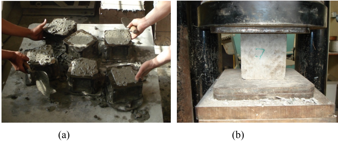
Figure 3.6: (a) Preparation of Cubes and (b) Cube test.
