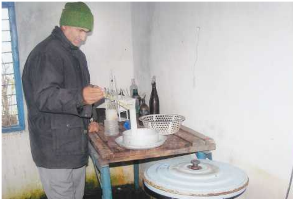
Checking of water portion of milk by Lato meter drop in the full milk of Lactojar there is also confituse machine to checking the fat of milk
