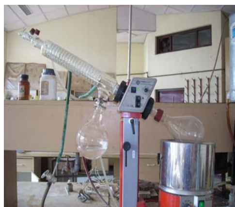
Plate 1 D: Concentration of solvent extract of A. dubia using rota – vacuum evaporator
