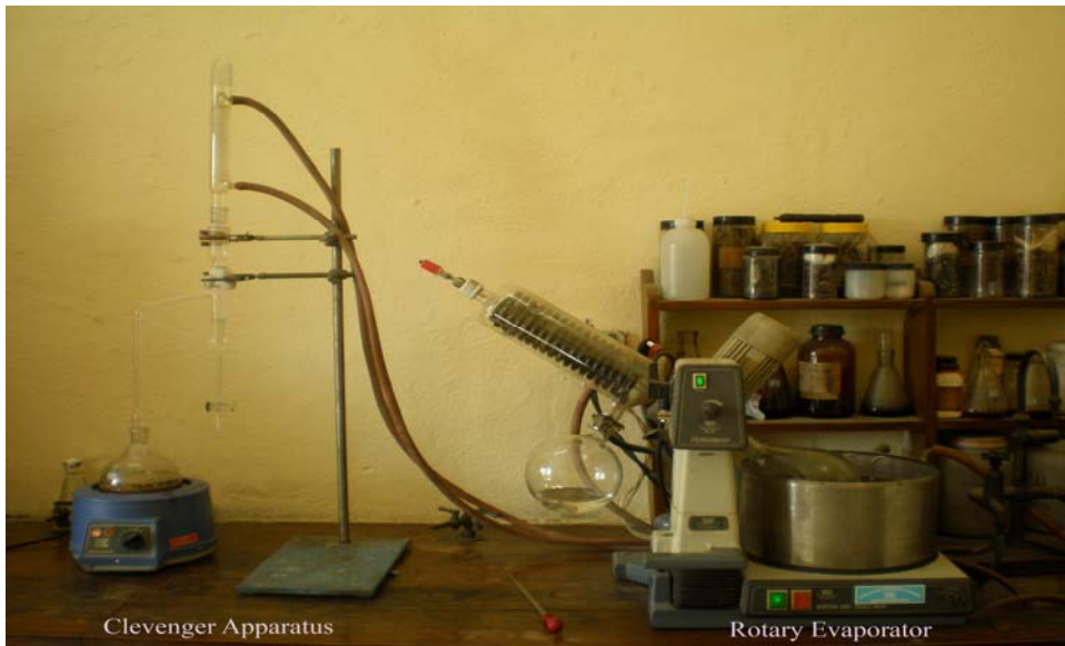
Photograph 3: Clevenger Apparatus and Rotary Evaporator
