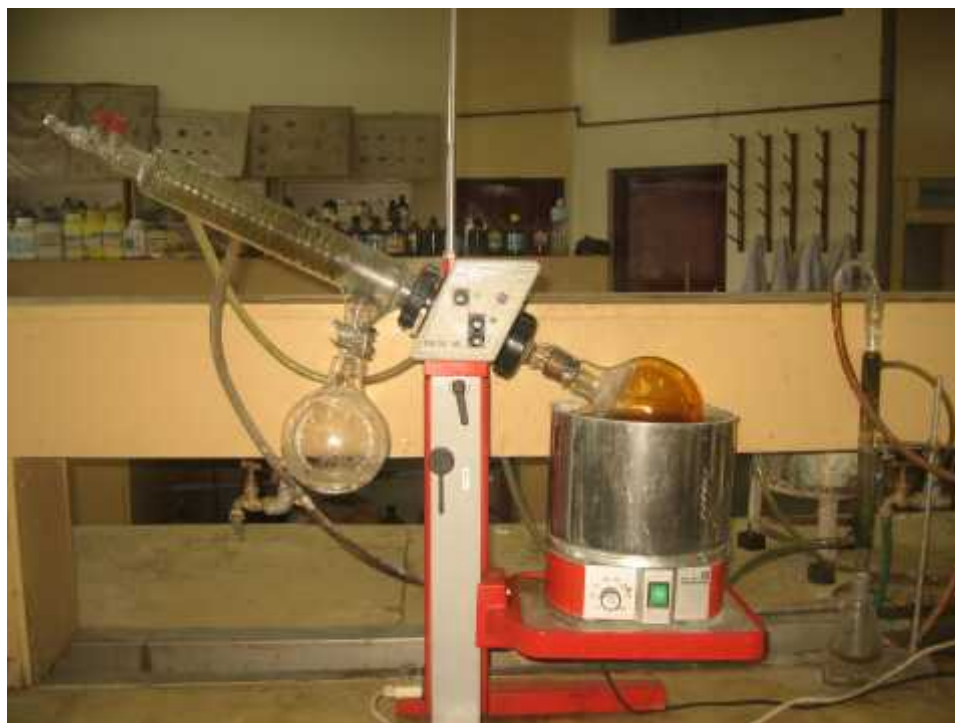
Photograph 2: Rotary vacuum evaporator showing the recovery of extracting solvent
