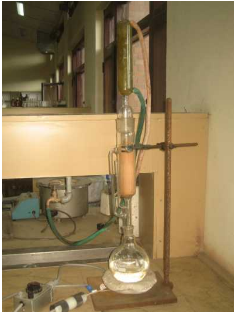
Photograph 1: Soxhlet extractor showing extraction of medicinal plants
