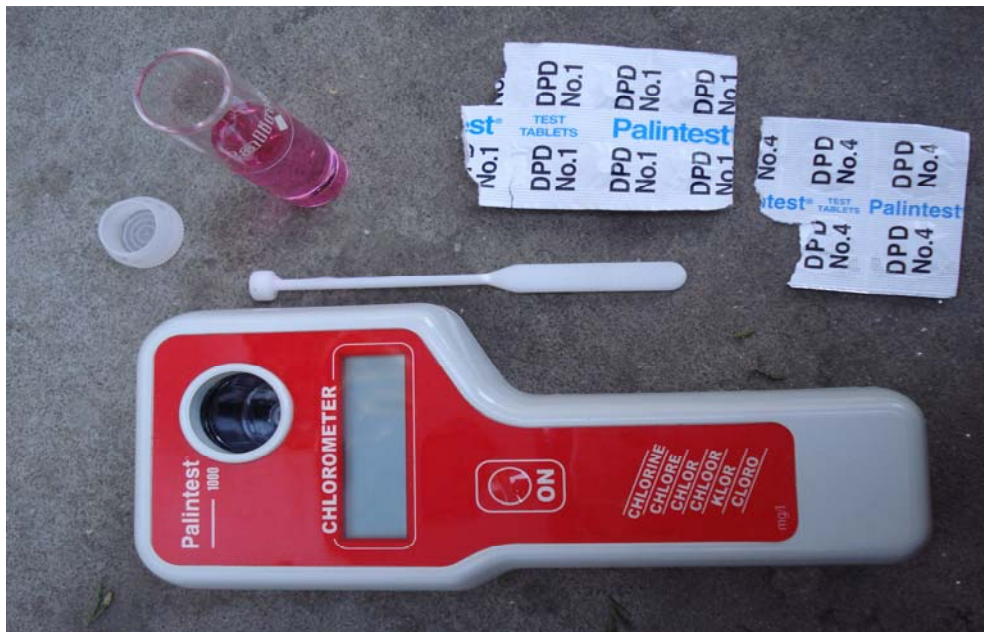
PHOTOGRAPH 2 : Chlorine determination by CHLOROMETER
