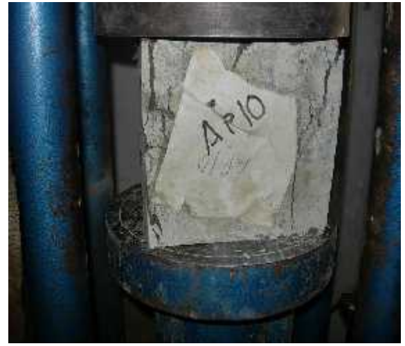
Fig 4.7: Failure Mode of Concrete Cubes under Compressive Loading
