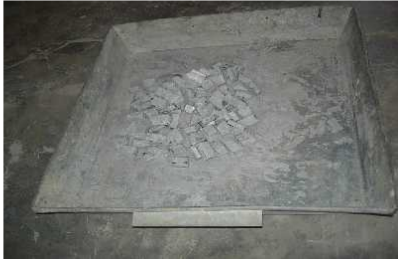
Fig. 3.2 Rubber Aggregate Coated with Cement
