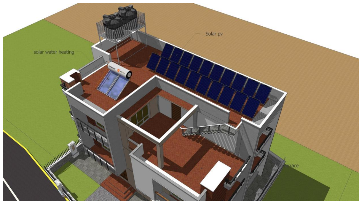
Figure 40: Typical Model House for Solar home installation
