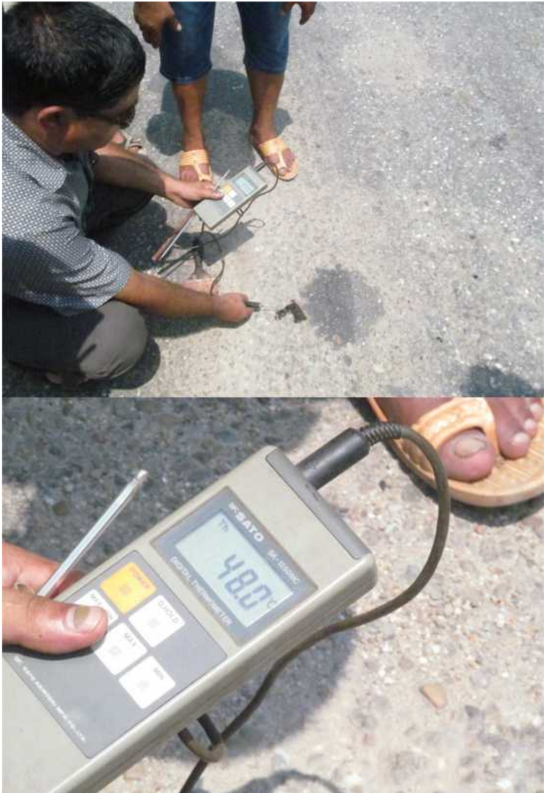
Figure 18 Recording Pavement Temperature
