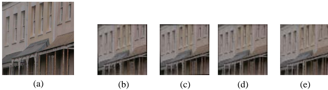
Figure B.2: Original and transformed images (a) HR image (b) down sampled, no transformation (c) 0^\circ , (0.479, 0.911) pix (d) 0.9^\circ , (0.737, 0.802) pix (e) 1^\circ , (0.123, 1.019) pix LR images
