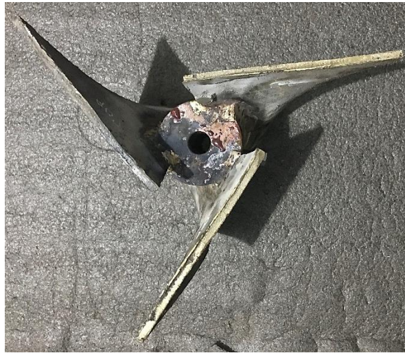
Figure 3.30 Final casted runner after gas welding
