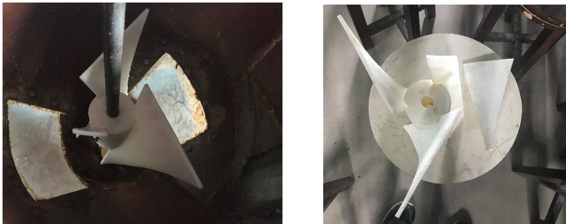
Figure 3.27 Broken runner during experiment
