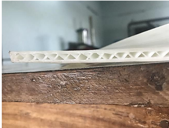
Figure 3.28 Weak infill of the material during 3D print
