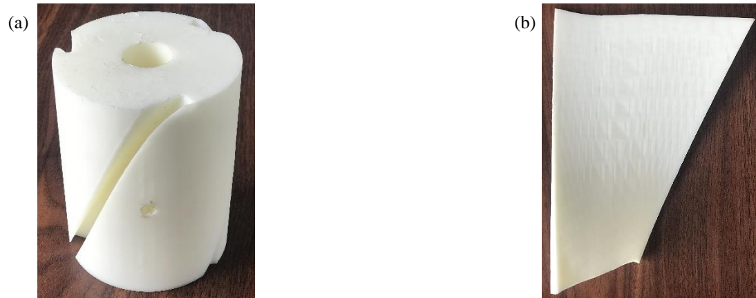
Figure 3.24 Fabricated runner parts (a) hub & (b) blade
