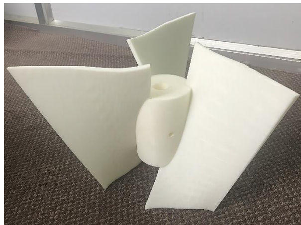
Figure 3.25 Assembled fabricated runner
