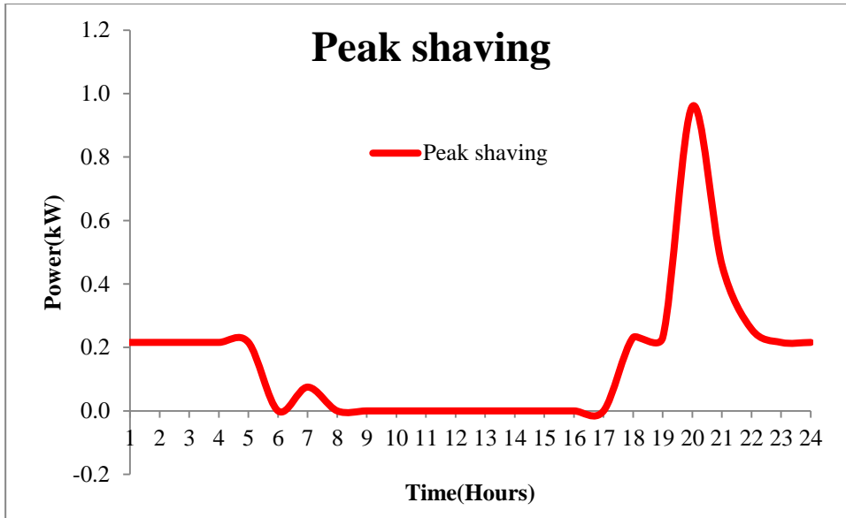
Figure 4.46: Peak shaving achieved after system installed for weekend for type 1 Here in the figure we can observe the maximum peak shaving of 0.95 kW at 8 pm for weekdays and weekend. The peak shaving is the energy that is supplied by battery which when in absence of battery must be supplied from grid.
