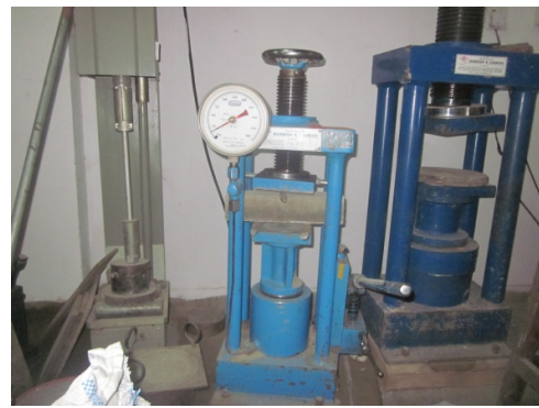
Compression testing Machine
