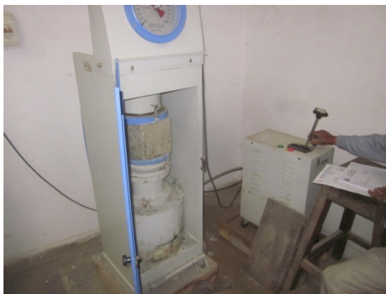
Compressive Strength Testing
