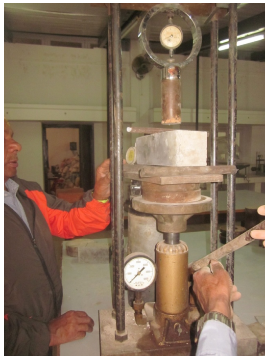
Figure 11: Flexural strength testing of concrete containing different percentage of plastic pet bottle fiber.
