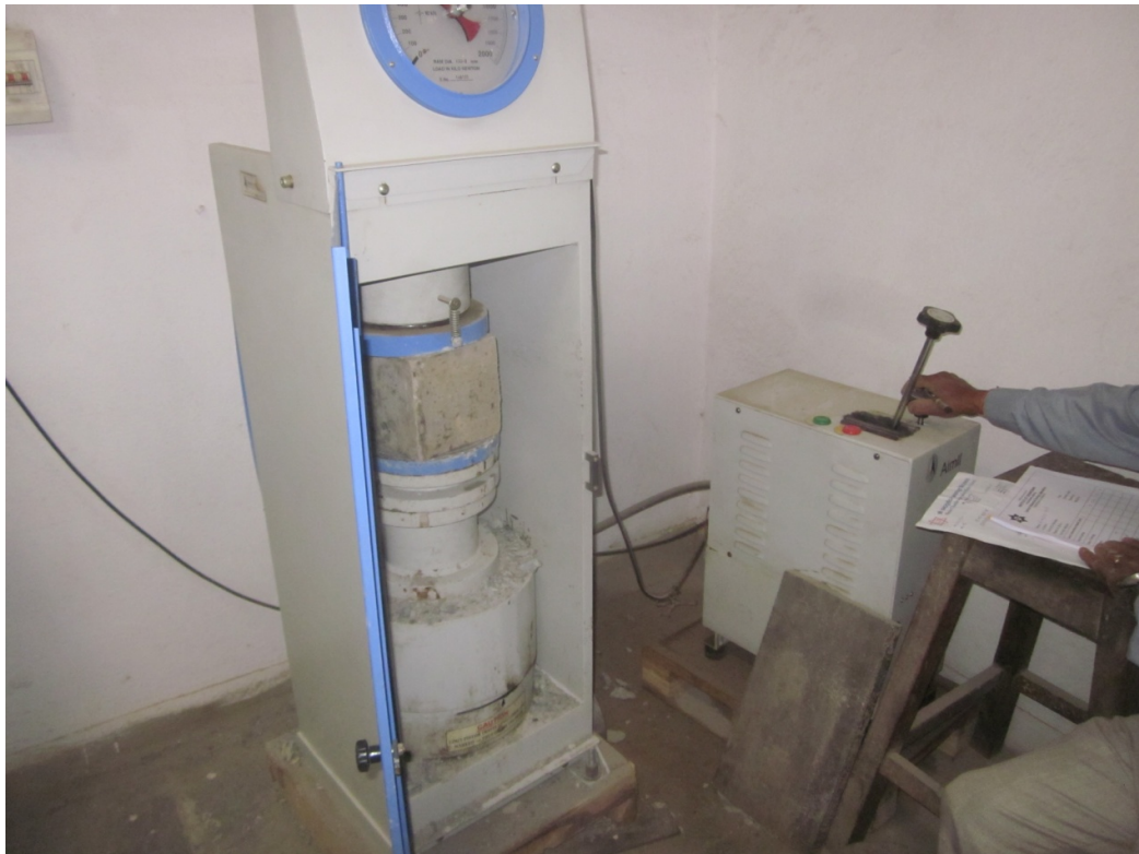
Figure 7: Compressive strength testing of concrete containing different percentage of plastic pet bottle fiber.
