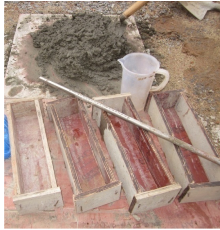
Beam Sample Preparation
