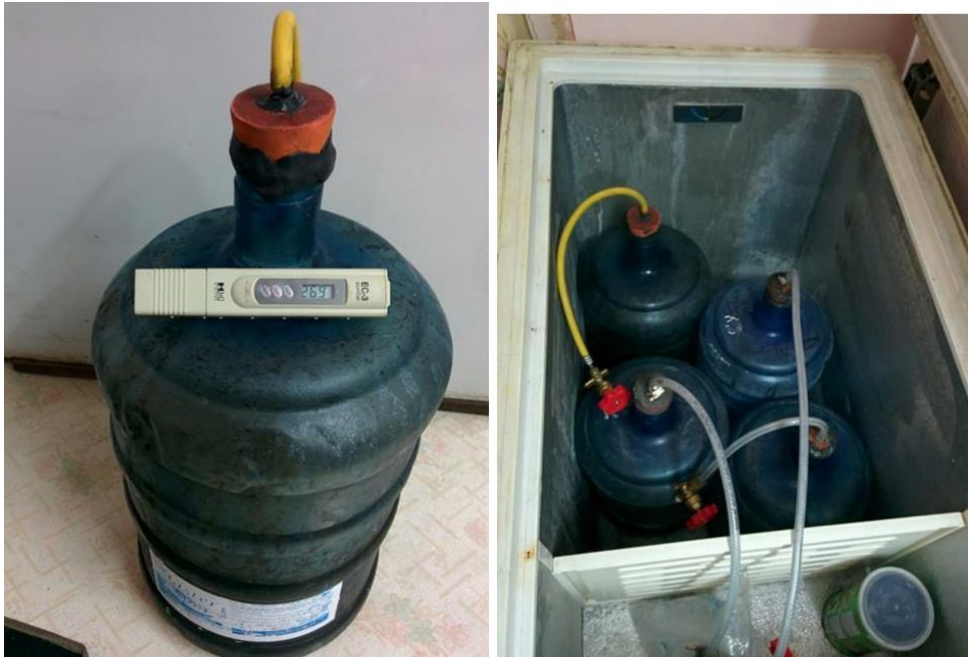
Prototype Digesters at room temperature and at low temperature inside refrigerator
