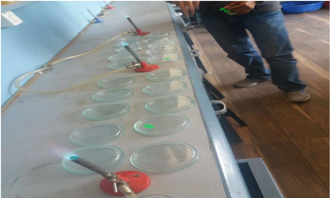
P1: Preparation of NA plate
