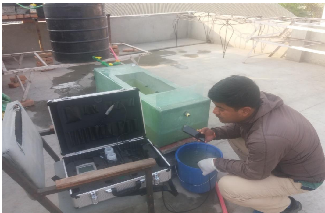
P6: Determination of water characteristics using conductivity meter and pH meter
